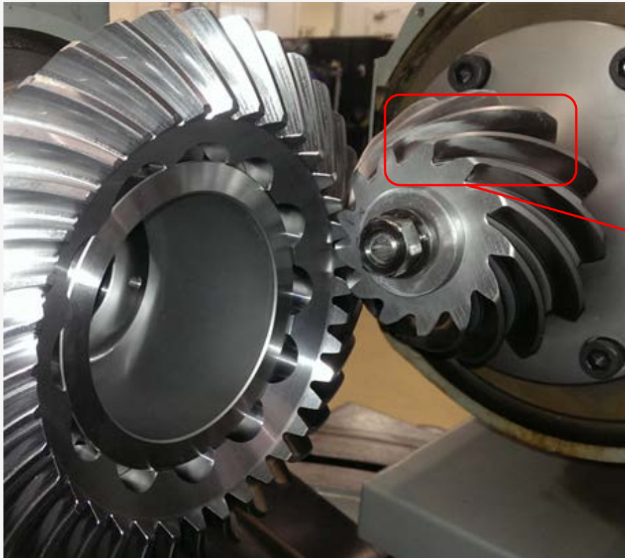
13x37 hypoid gear pair on the VH tester
